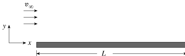
Figure 3.1. Flow on a flat plate.
