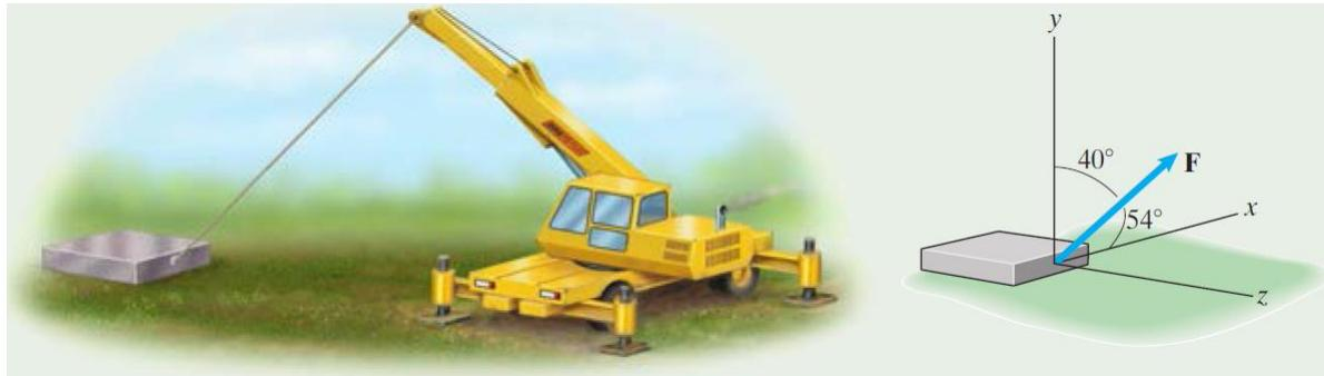
**Determining Components in Three Dimensions.** The crane exerts a 600-lb force  $\mathbf{F}$  on the caisson. The angle between  $\mathbf{F}$  and the  $x$  axis is  $54^\circ$ , and the angle between  $\mathbf{F}$  and the  $y$  axis is  $40^\circ$ . The  $z$  component of  $\mathbf{F}$  is positive. Express  $\mathbf{F}$  in terms of components.
